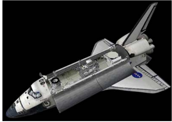
Image 1: Graphical overview of the payload bay configuration of Space Shuttle Endeavour for STS-134 with the Orbiter Docking System (ODS) in the front, the EXPRESS Logistics Carrier (ELC)-3 in the middle and the Alpha Magnetic Spectrometer (AMS)-02 in the rear (Credit: NASA).
