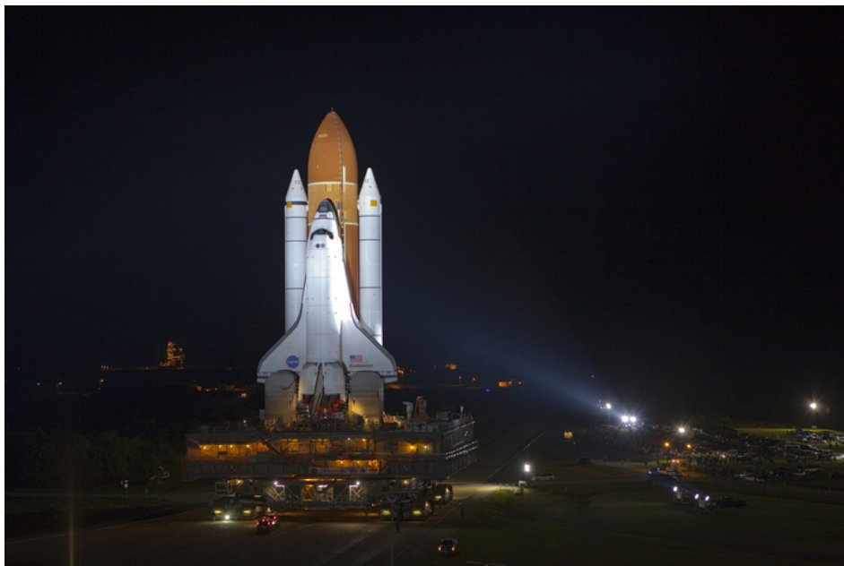
Image 2: Space Shuttle Endeavour rolls out of the Vehicle Assembly Building (VAB) on 10 March 2011 on its way to launch complex 39A. The Shuttle stack, composed of the Orbiter, the orange External Tank and two Solid Rocket Boosters, stands on its launcher platform, which itself is carried by one of the Crawler Transporters.
