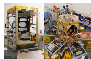
Sentinel-5P : Raw structure (left) and equipped (right). ©APCO (left), ADS (right)
