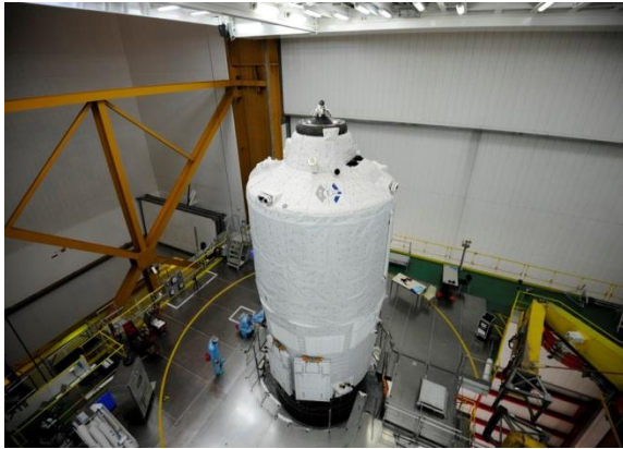
Installation of ATV-5 Georges Lemaître on Ariane 5 ES launcher at the satellite preparation complex Guiana Space Centre in Kourou, French Guiana. (Photo: ESA).
